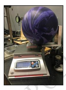
2. Place the bowling ball in the cradle so the CG is aligned with the marking on the right edge of the frame's arm and the pin is aligned with the cradle arm facing upwards. Press "Tare" on the scale to zero out the reading.
