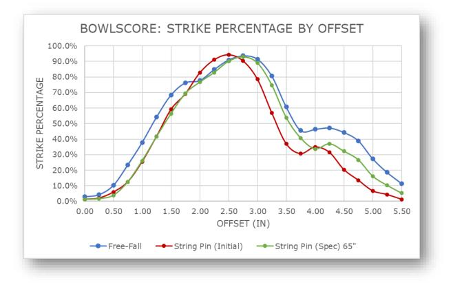
Applying the same analysis to the data from the new machines that meet the preliminary specifications, we still see a reduction in striking on the very high and low ends of the pocket. Overall, the data has moved closer to the behavior of our free-fall control set. The previous difference of 10.7% has been reduced to 7.1% -- a percentage difference of about 34% closer to free fall.
