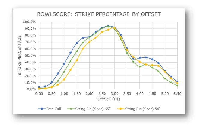
We can see that shortening the strings from 65" to 54" in our Bowlscore testing minimally impacted the striking profile of the pinsetters. This was expected, as the first-ball cycle has typically been less affected by the string lengths than the second-ball cycle.
