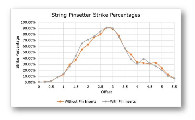
The results showed that bowling with or without the pin inserts resulted in little to no change in the pin performance. Additionally, some of the metal inserts wore down on the strings to the point that the strings would break during testing.
