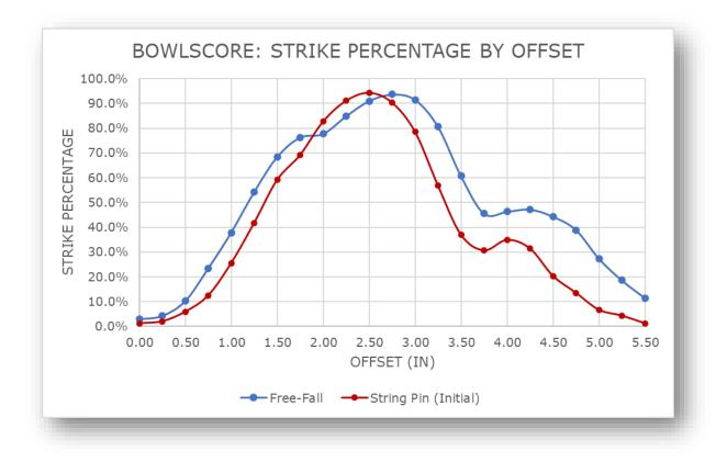
In our original testing, we saw offsets where strings struck more, and offsets where they struck less. Cumulatively we saw approximately a 10% decrease in striking when going from free-fall to strings.
