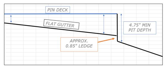
It is important to note that, during the retesting, we came exceptionally close to having the 10 pin return up the flat gutter on the 7-pin side. But, so far in our additional testing, we have not converted any challenging splits due to rebounds.
