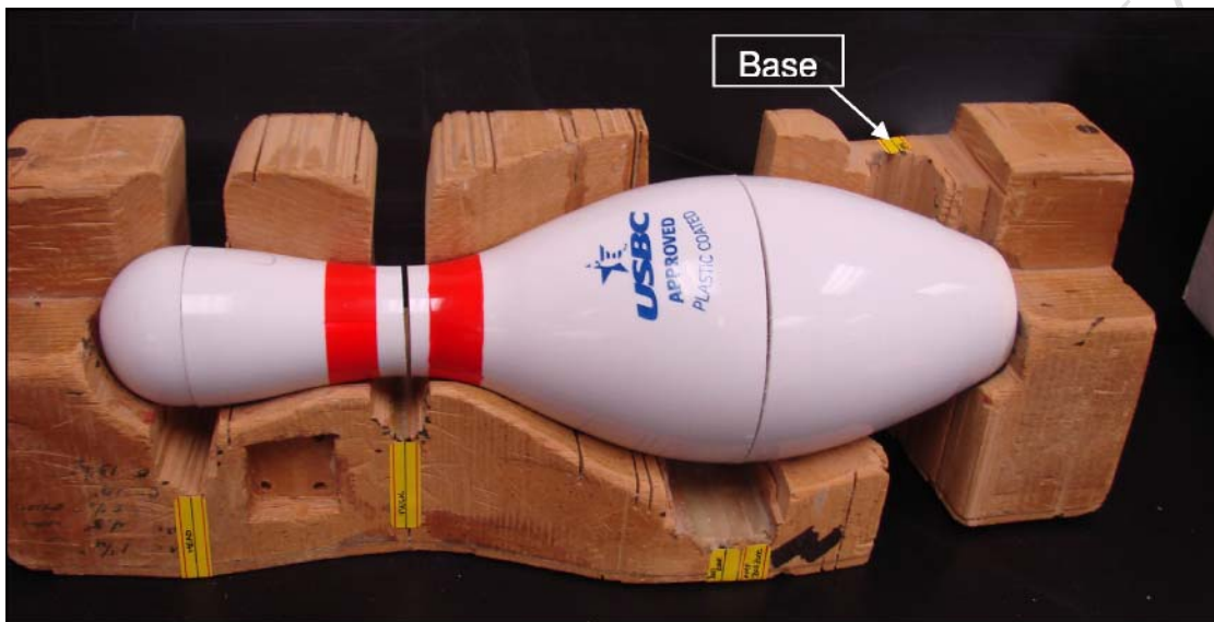
Figure 2 – Cut bowling pin in the cutting jig. The cut made with the jig at this position is the cut at the base of the bowling pin.
